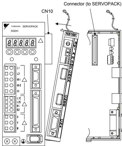
3. For grounding, connect a ground wire of the NS100 Module to the marked “G” on the SERVOPACK.
