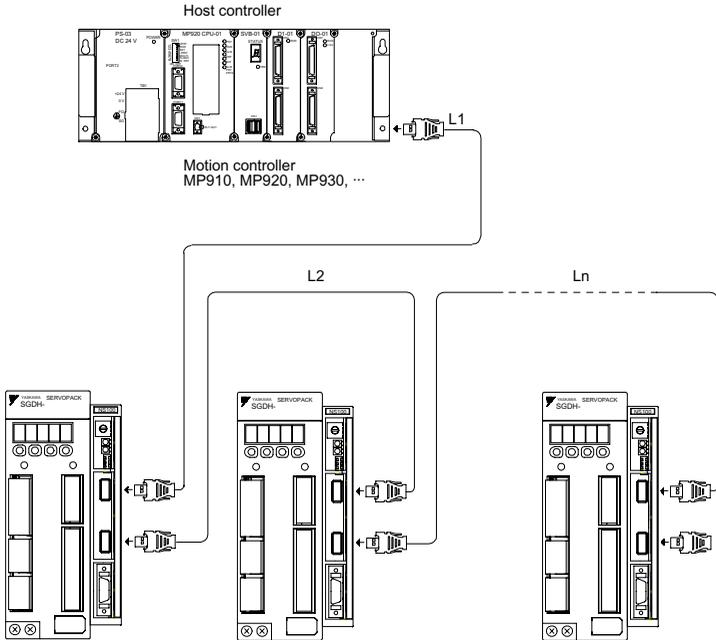
Note: The total length of cable should be “ $L1 + L2 + \dots + Ln \leq 50m$ ”
