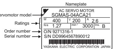
Note: Contents of the nameplate may differ in accordance with the series or type of the motor.
