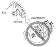
When you attach the coupling, do not subject the shaft to shock.
