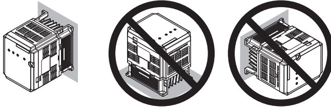
Figure 8 Correct Installation Orientation (Braking Unit)
