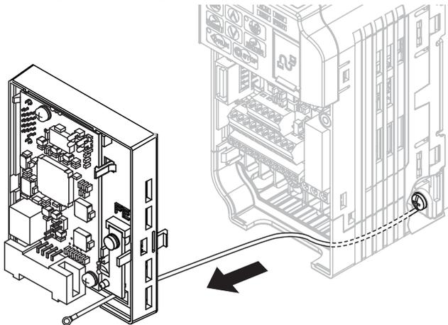
**Figure 15 Ground Wire Routing**
