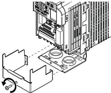
**Figure 8 Remove the NEMA Type 1 Terminal Cover**
