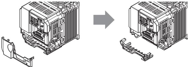
**Figure 6 Remove the Terminal Cover and Bottom Cover on an IP20/Open-Chassis Drive
