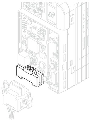
Figure 3 Communication Cable Connector
