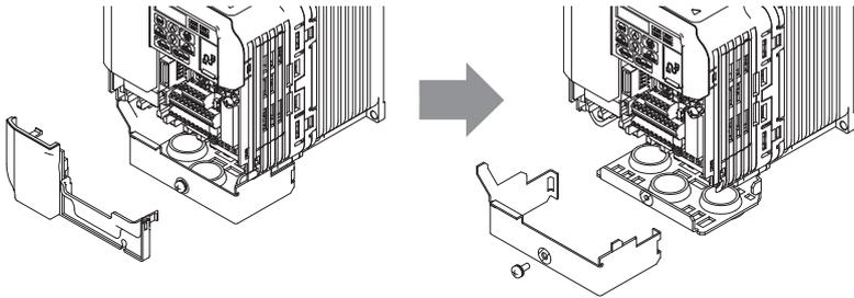
**Figure 9 Remove the Terminal Cover on an IP20/NEMA Type 1 Drive
