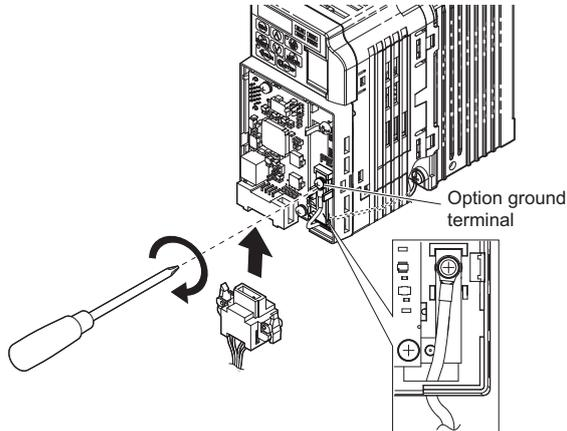
Figure 17 Connect the Ground Wire and CompoNet Cable Connector to the Option
