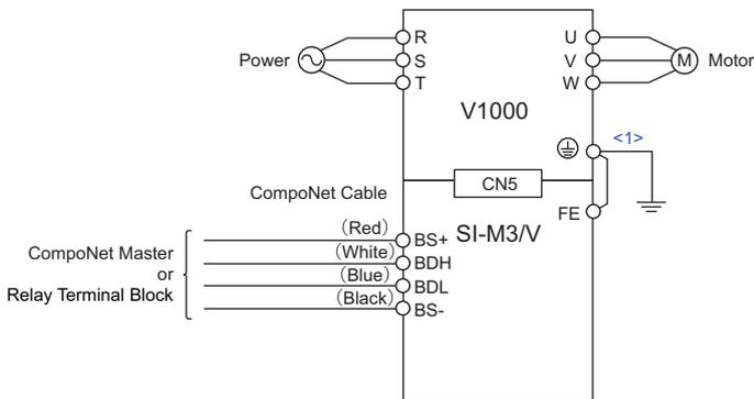
Figure 18 Wiring Diagram
