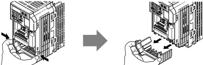
**Figure 5 Remove the Bottom Cover on an IP20/Open-Chassis Drive
