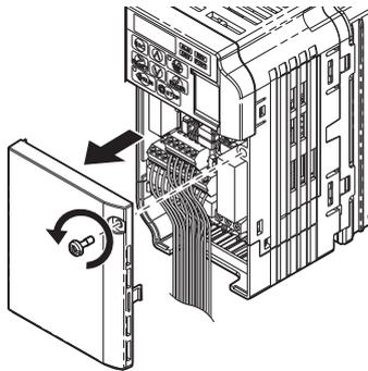
Figure 4 Remove the Front Cover
