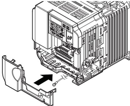
Figure 13 Reattach the Terminal Cover
