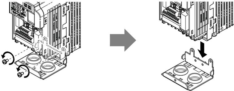
**Figure 10 Remove the NEMA Type 1 Conduit Bracket**
