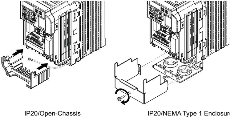
Figure 12 Reattach the Bottom Cover
