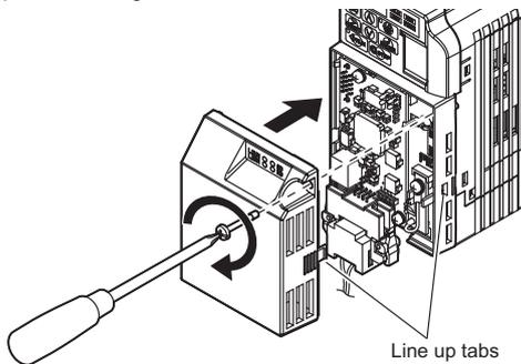
Figure 19 Attach the Option Cover
