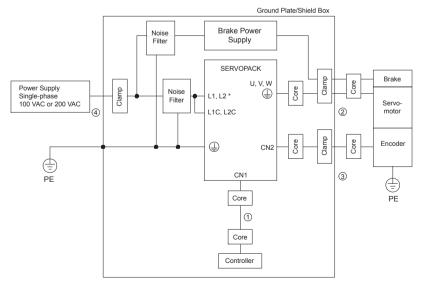
Connect main power supply to terminals L1-L3 for SGDH-08AE-S and SGDH-15AE-S.
