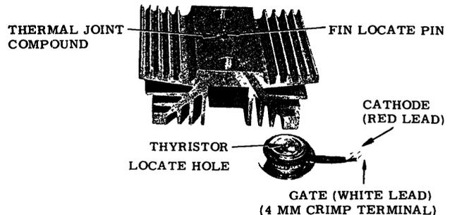
Fig 21 View After the Removal of Thyristor
