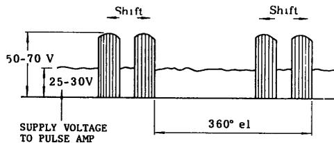
Fig. 25 PS Output Waveforms
