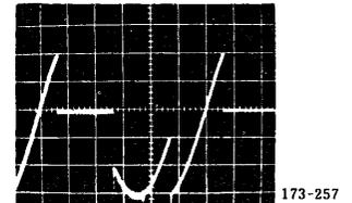
Fig 27 Thyristor Voltage Waveforms across Terminals A-K
