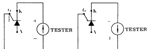
( IF TESTER READING IS ZERO OR  $\infty$  ON EITHER ONE OF TWO MEASUREMENTS THYRISTOR MODULE IS DEFECTIVE )
