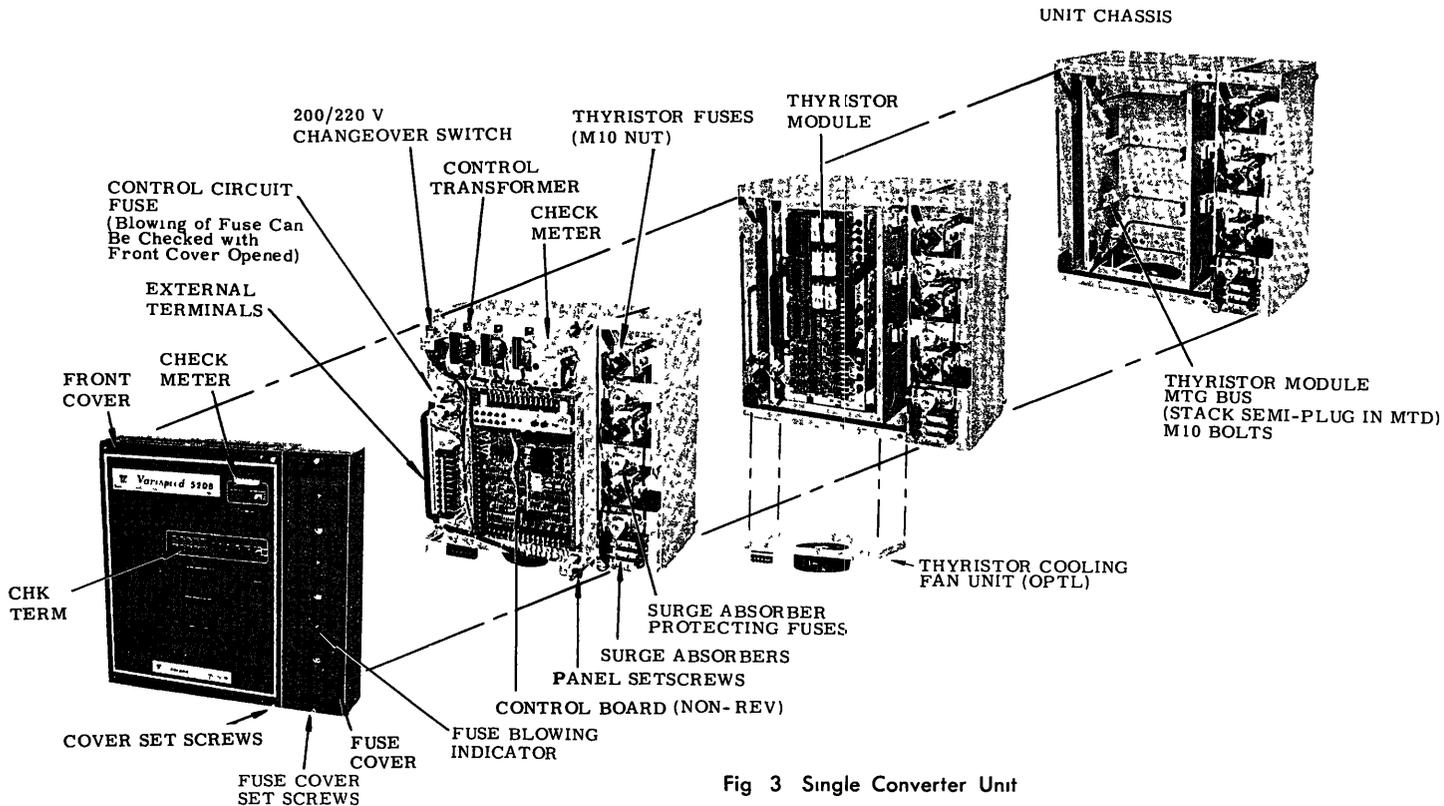
Fig 3 Single Converter Unit
