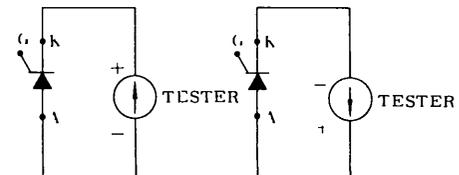
( IF TESTER READING IS ZERO ON EITHER ONE OF TWO MEASUREMENTS THYRISTOR MODULE IS DEFECTIVE )
