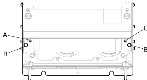
Figure i.32 EMC Filter Switch Location (2A0075 to 2A0114, 4A0052□□A, and 4A0065 to 4A0096)
