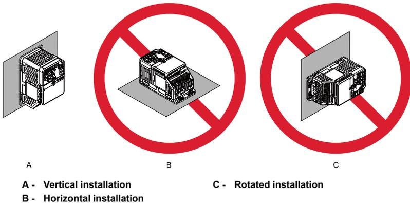
**Figure 9.4 Installation Orientation**
