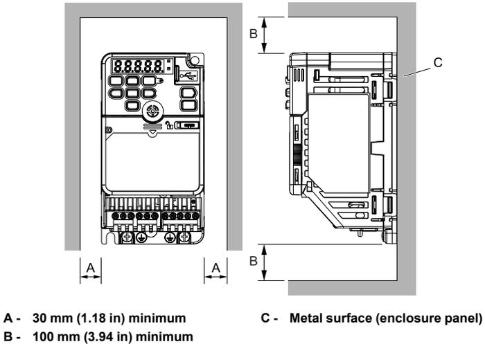
**Figure 9.5 Installation Clearances**
