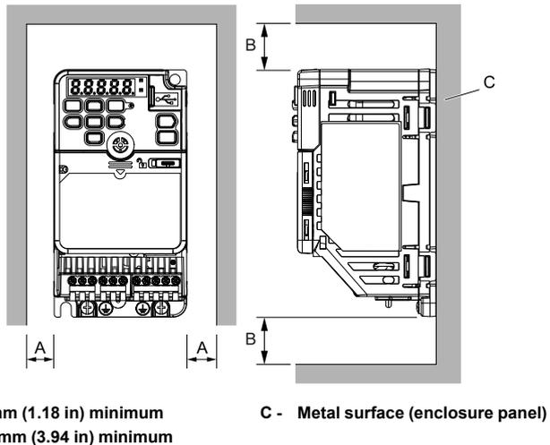
Figure 7.3 Installation Clearances
