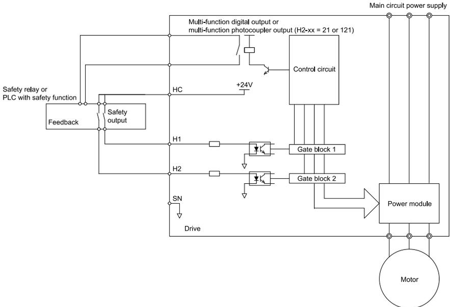
**Figure 20.2 Safe Disable Function Wiring Example**
