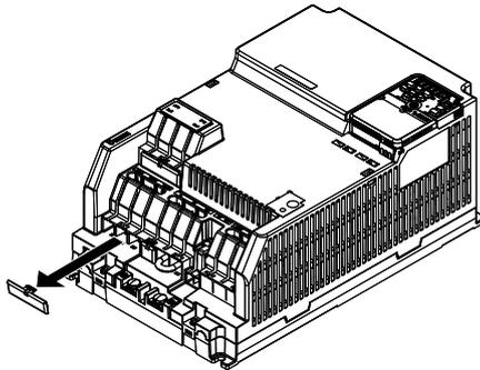
**Figure 10.7 Remove IP20 Terminal Protective Cover**
