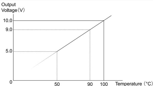
**Figure 7.2 Heatsink Plate Temperature Output on MFAO**
