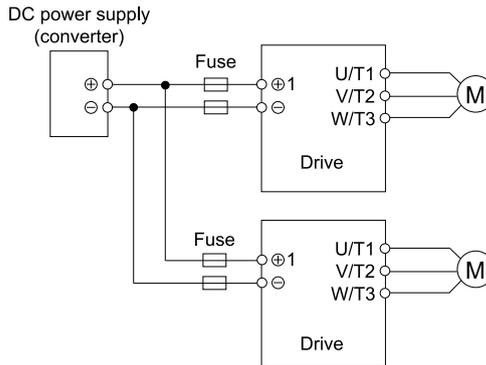
Figure 16.3 Wiring Example for DC Power Supply Input
