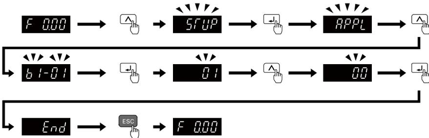
**Figure 12.2 View and Set the Necessary Parameters**
