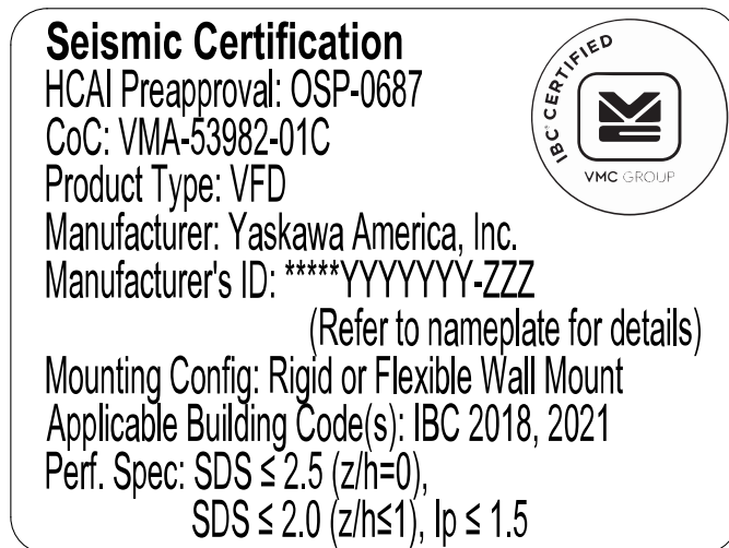
Figure 18.1 Seismic Certification Label Example for Drives
