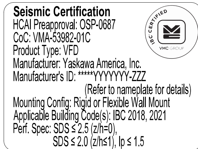
Figure 18.1 Seismic Certification Label Example for Drives
