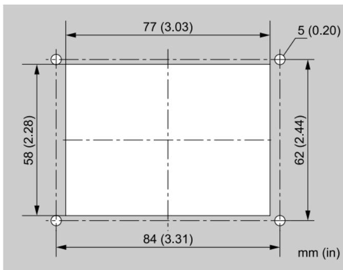
Figure 5.2 Panel Cut-out Diagram
