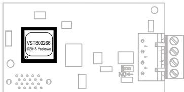
Figure 2 Option Card Software Version Location
