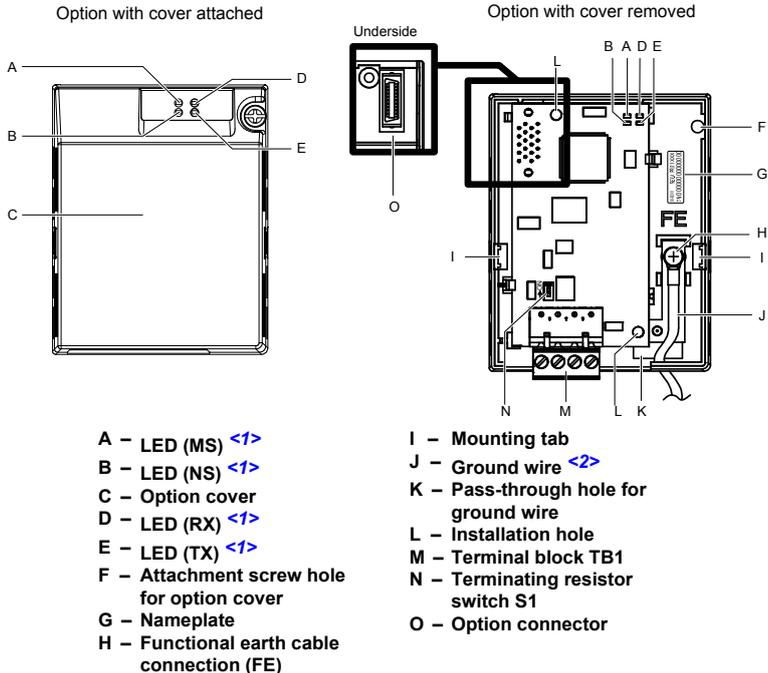
Figure 1 Option Unit Components
