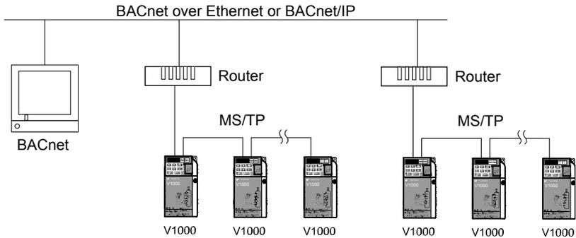
**Figure 20 Connecting Multiple Drives to a BACnet Workstation – System Overview**
