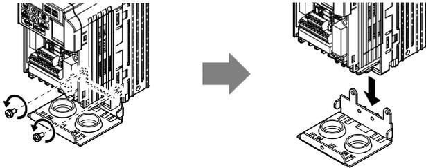
**Figure 10 Remove the NEMA Type 1 Conduit Bracket (Models BA0001F to BA0003F and 2A0001F to 2A0006F)**
