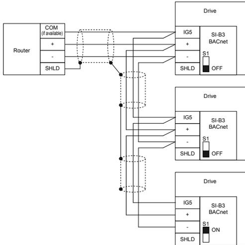
**Figure 19 Connection Diagram for Multiple Connections**
