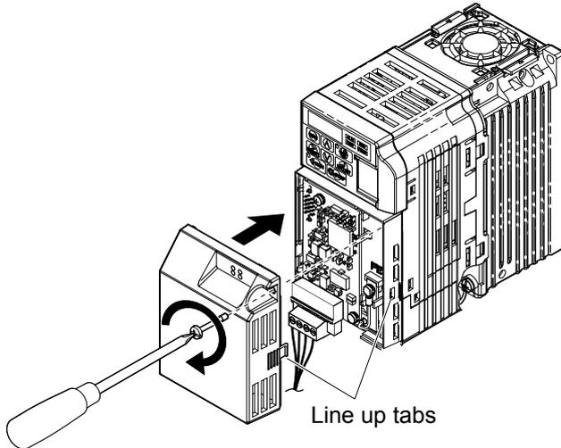
Figure 21 Attach the Option Cover
