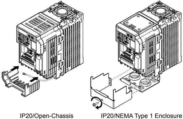
**Figure 12 Reattach the Bottom Cover**
