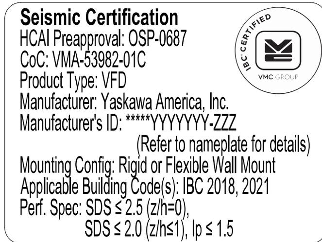
**Figure 2.1 Seismic Certification Label Example for Drives**
