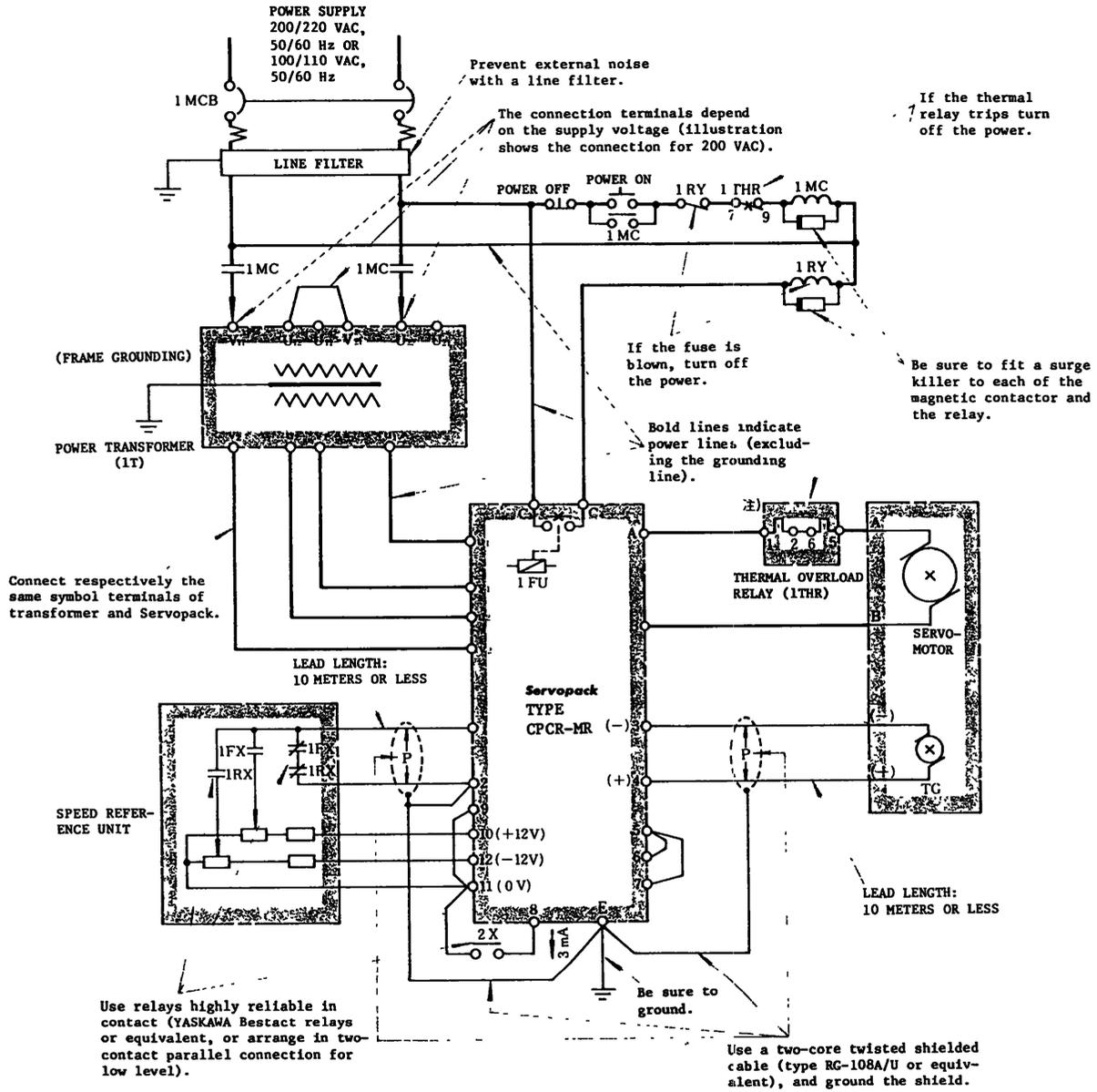
Note: The thermal overload relay (1THR) for PM or JM provides neither terminal 5 nor 6.
