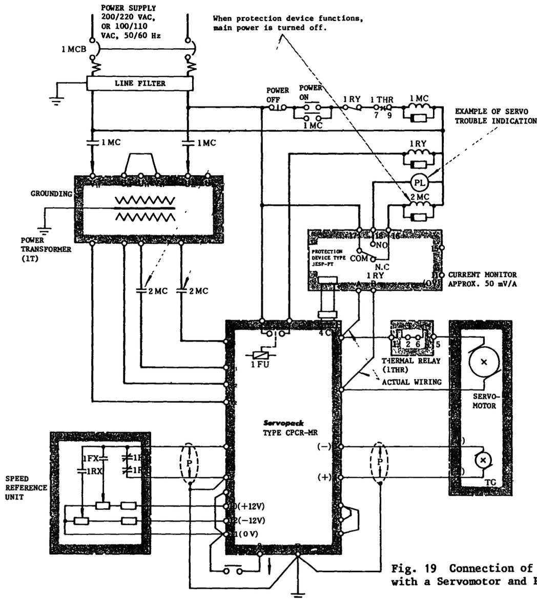
**Fig. 19 Connection of Servopack with a Servomotor and Peripherals**
