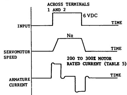
Fig. 8 Servomotor Start-Stop Characteristics
