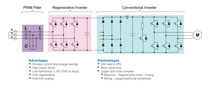
An AFE saves energy by putting the regenerative energy back onto the line. However, unlike an FFE, an AFE uses a PWM waveform to regenerate back onto the line.
