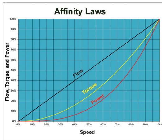
Figure 4: Affinity Laws show that Flow \propto Speed / Torque \propto Speed^2 / Power \propto Speed^3
