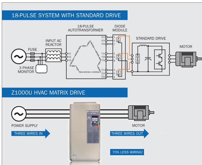
Comparison of 18-pulse drive system with Z1000U HVAC Matrix drive system
