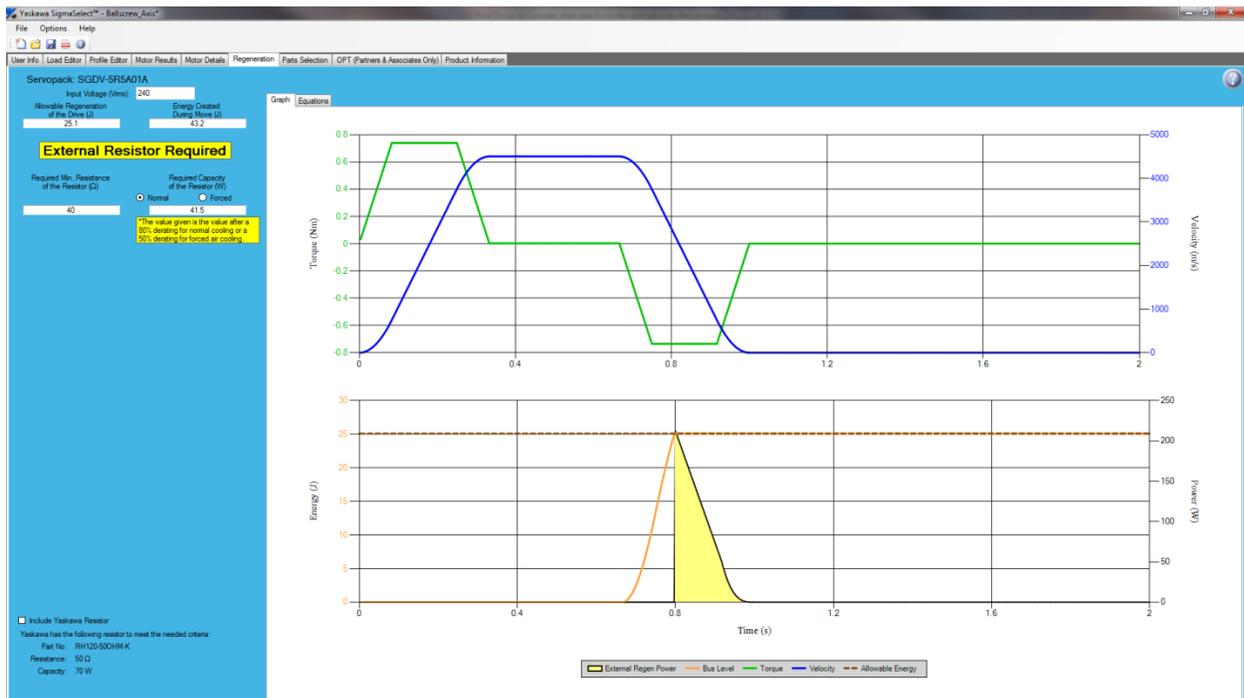
Figure 3: Calculations may show that an external regeneration resistor is required when using the Yaskawa SigmaSelect servo sizing software.
