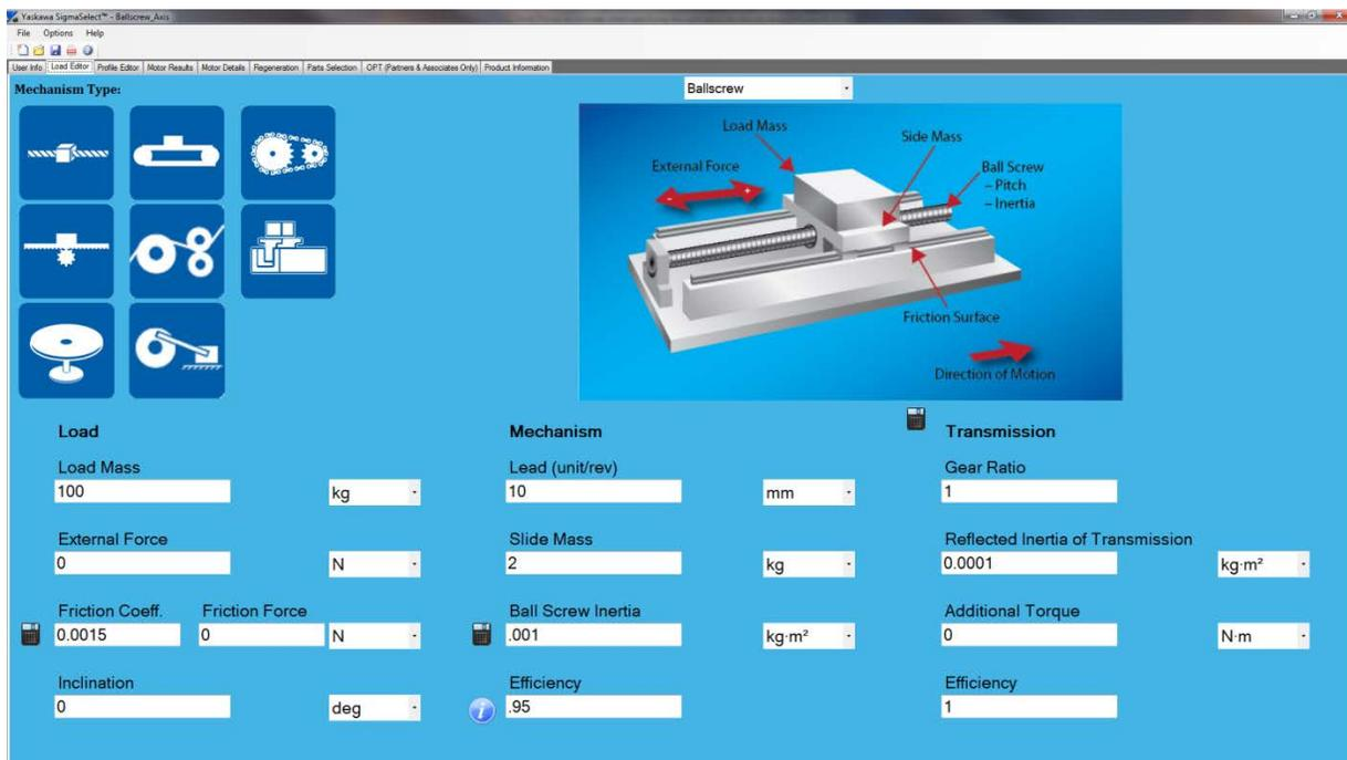
**Figure 1: Software can help in sizing a servo system. This typical load/mechanism entry screen from Yaskawa SigmaSelect servo sizing software shows a diagram calling out external force, load mass, side mass, pitch, and inertia of the ball screw, friction, and motion direction.**
