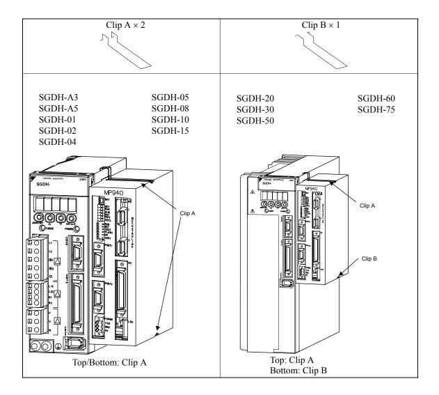
3. Insert the mounting clips into the mounting holes in the MP940, as shown in the figure below.
