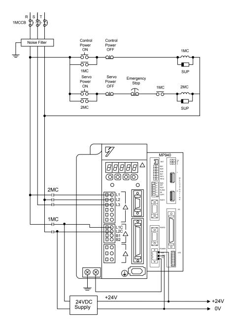
Figure 2.9: Three-phase Wiring
