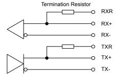
Figure 5.4: Internal Termination Resistors
