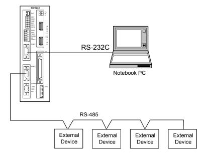
Figure 5.3: Branched Connection of Peripheral Devices
