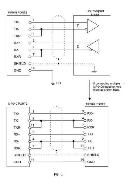
Figure 5.5: Wiring Diagram
