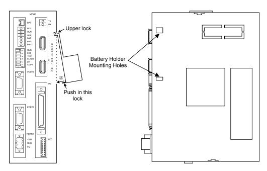
Figure 2.4: Mounting the Battery Holder
