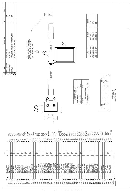
Figure 13.4: I/O Cable Drawing
