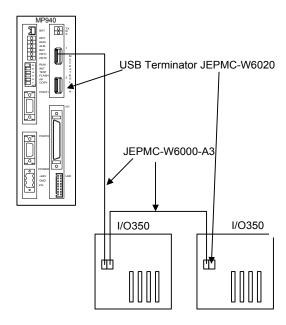
Figure 5.7: MP940 Connection to Multiple I/O 350 Modules
