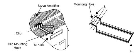
Figure 2.3: Inserting the Mounting Clips
