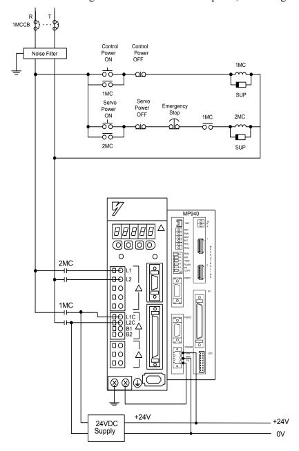
Figure 2.8: Single-phase Wiring
