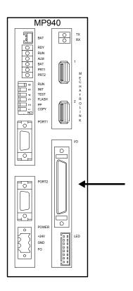
Figure 6.1: Digital I/O Connection
