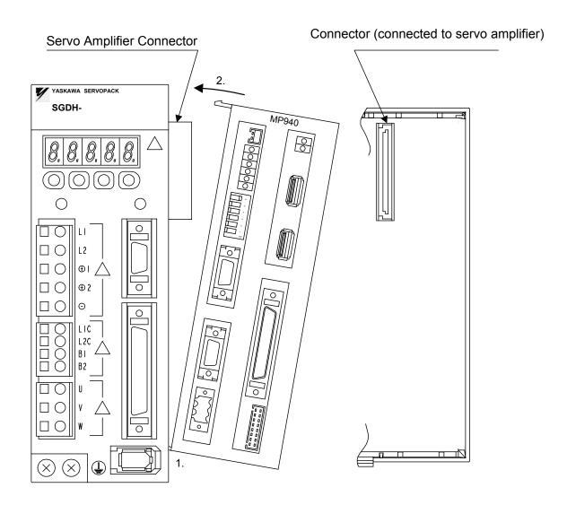
Figure 2.2: Mounting the MP940 to an SGDH Servo Amplifier
