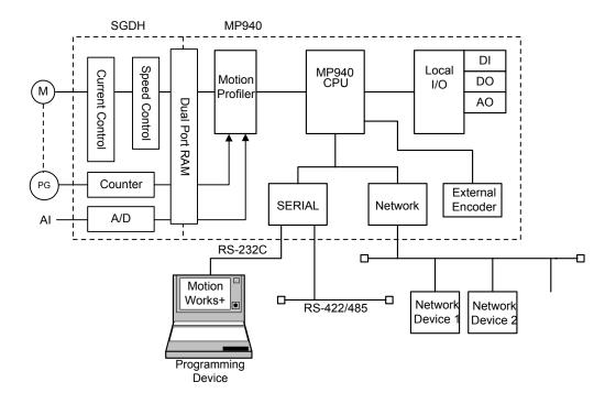
Figure 1.2: Block Diagram of MP940 Functions
