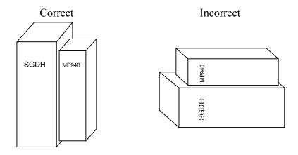
Figure 2.1: Mounting Orientation
