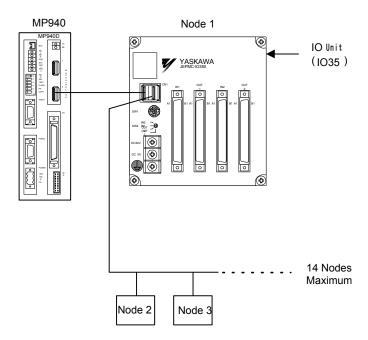
Figure 5.6: Mechatrolink Connection Example
