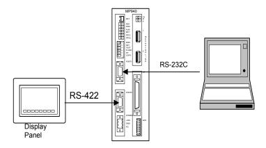
Figure 5.2: Serial System Configuration
