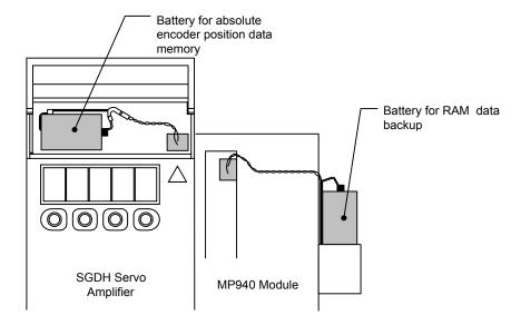
Figure 2.6: MP940 and SGDH Batteries
