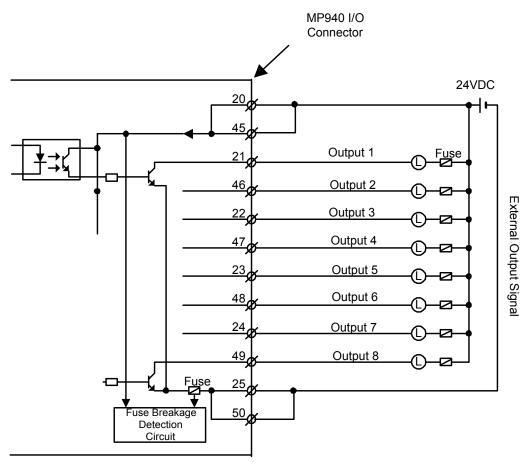
A fuse is included on the common output line of the MP940 module as a protection circuit. However, there is a risk of the fuse not breaking due to an external short. Provide an external 100mA fuse on each output for added protection.
