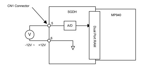
Figure 8.1: Analog Input Data
