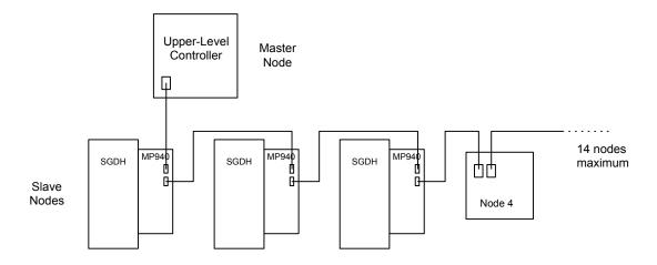
The MP940 cannot communicate directly to the I/O350 or distributed I/O if configured as a slave.
