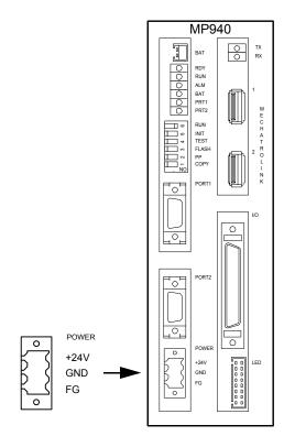
Figure 2.7: MP940 Power Connection
