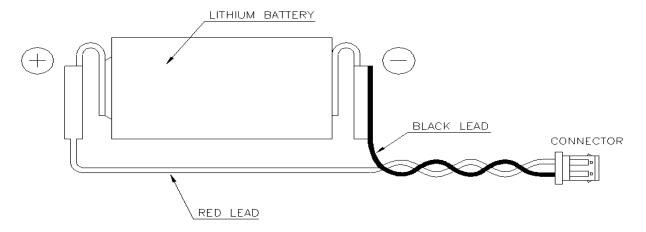
Figure 11.1: BA000518 Battery with Cable
