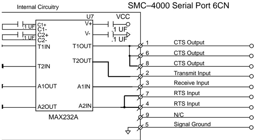
**NOTE: Hardware handshaking must be used with the SMC-4000. If it is impossible to implement hardware handshaking, use a jumper between pins 1 and 4 in the connector.**
