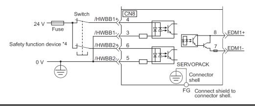
(10) Cable with Connector for CN8 (Model: JZSP-CVH03-03-E)
