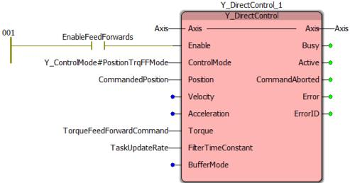
(Note: with a tightly tuned servo, if the torque feed forward leads to a large position error the servo loop gains will take control and ignore the torque feed forward input to maintain position control)
