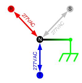
wye configuration with the neutral grounded in order to limit voltage to 277V or less to ground.
