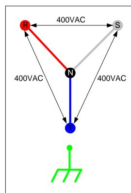
The 5 wire system is used to get balanced 400 V phase to phase and 230V phase to neutral (400/1.732) so control voltage can be obtained without a control transformer.
