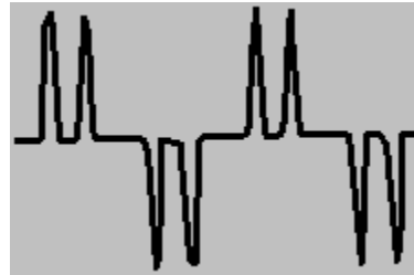
Fig. 2 Actual input current waveform for six pulse VFD without any filtering.
