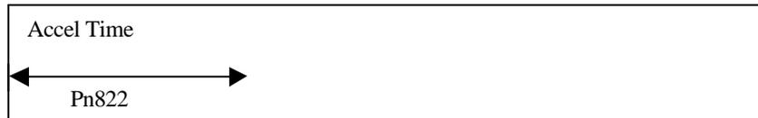
The same principal applies to the acceleration RATE for feeding (jogging) and homing. Use **Pn832** to set the acceleration time and define the acceleration rate for feeding (jogging). **Pn80A** sets the acceleration time and defines the acceleration rate for homing. All three acceleration time parameters work with the Maximum Feed Speed, Pn843.
