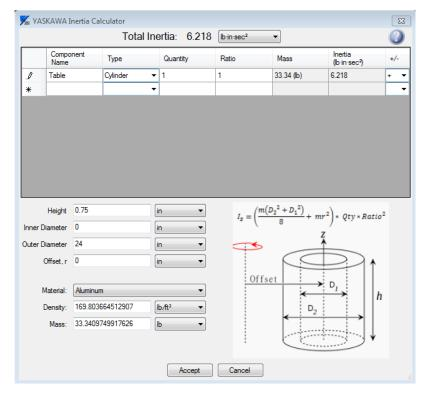
Next, subtract out the holes that are in the table. On the next row of the inertia calculator table, choose a **Component**Name of "Holes" and a **Type** of "Cylinder". Since there are six holes, change the **Quantity** to 6. Because the inertia of the holes is to be *subtracted* from the inertia of the table, change the +/- field to - (minus).
