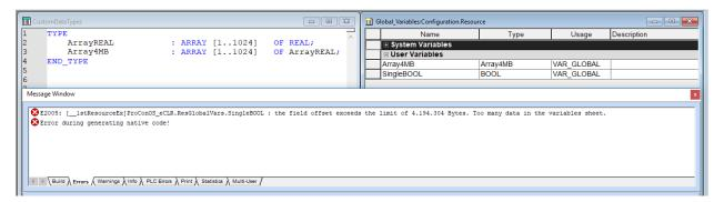
Compile without errors as long as the head address is declared inside the 4MB limit
