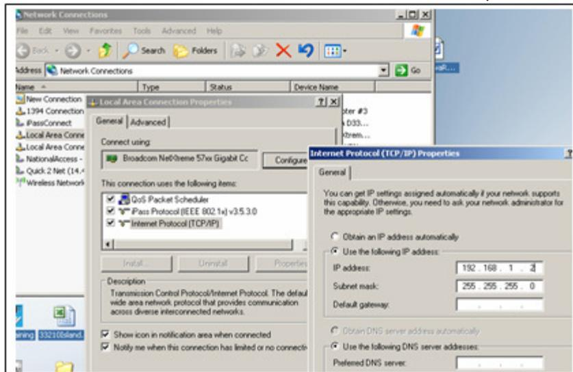
f) Connect to the controller using the Hardware Configuration. Confirm the IP address of the controller shows properly in the address fields and connect ONLINE. A confirmation message box will ask to use the configuration found during auto discovery. Click Yes.
