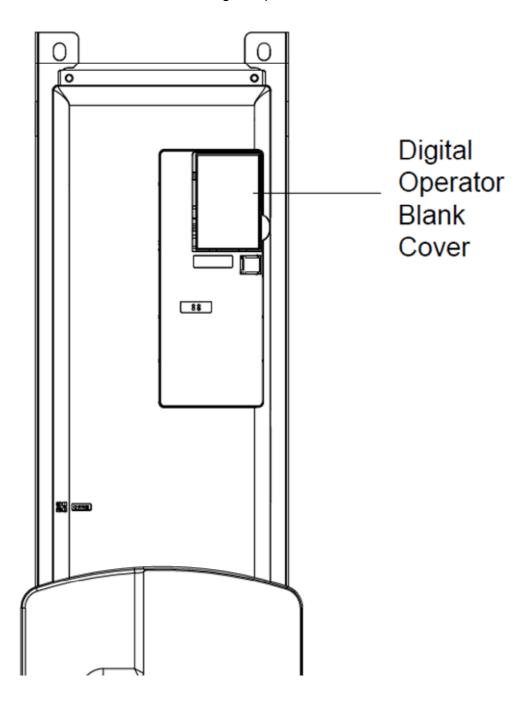
3. Disconnect the digital operator from the bypass portion of the cabinet.
