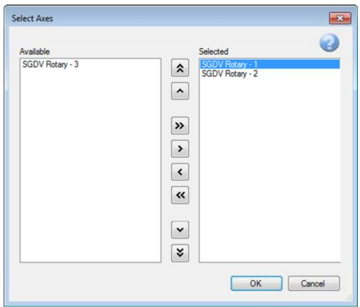
The order of the selected axes determines the column order in the parameter grid. Use the up and down arrows to change the column order. The double up and down arrows will move the selected axis to the top or bottom of the list.
