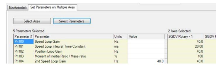
Notice that when the values do not match the value column is blank, which helps to quickly identify differences.
