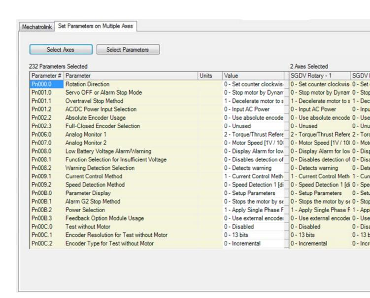
For ease of comparison, press the 'Select Parameters' button to choose a subset of the parameters to compare.
