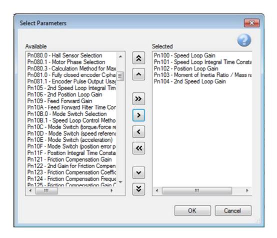
Similar to the 'Select Axes' dialog box, use the right and left arrows to select or remove parameters, and use the up and down arrows to change the order of the selected parameters.
