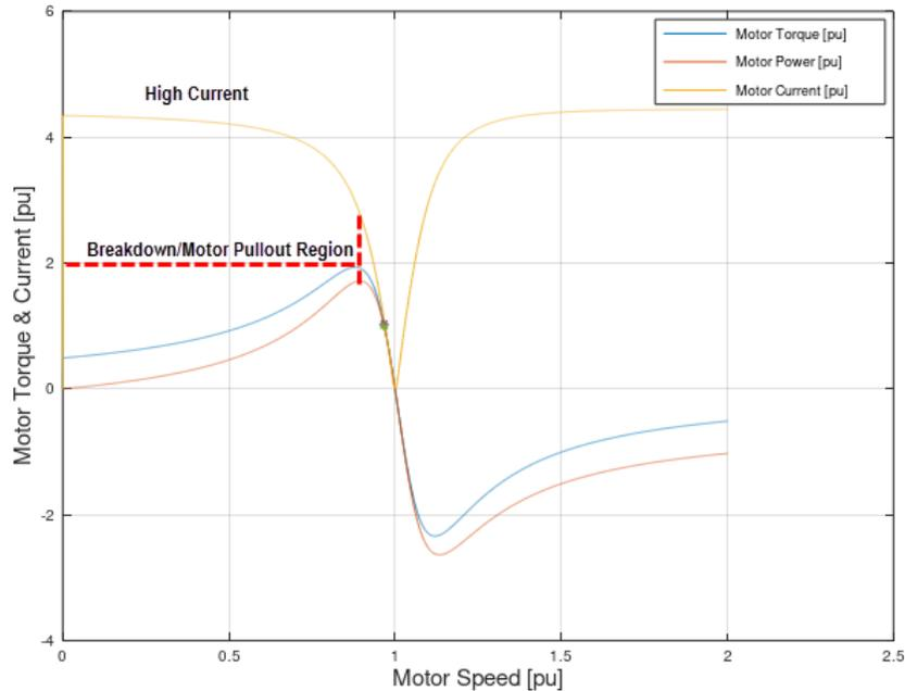
Figure 2: Normalized Power/Torque vs. Speed curve of a typical Induction Motor. If slip increases, operating speed falls into breakdown region, where motor pullout draws high current.
