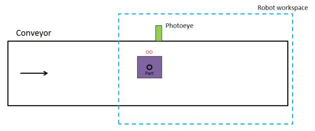
FIGURE 11 CONVEYOR MOVES PART DOWNSTREAM AND TRIGGERS PHOTOEYE AND REPRESENTS POINT OO
