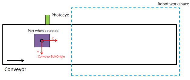
FIGURE 25 REPRESENTATION OF WHEN A PART TRIGGERS PHOTOEYE IN THIS SET UP
