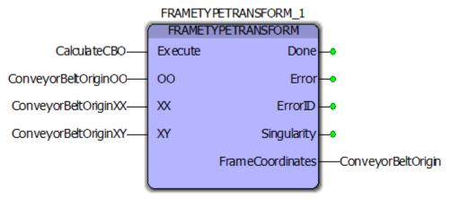
FIGURE 30 CALCULATE CONVEYORBELTORIGIN WITH FRAMETYPETRANSFORM IN MATH\_TOOLBOX
