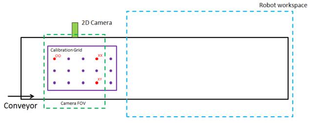
FIGURE 32 CALIBRATION GRID MARKED WITH OO XX XY PLACED OUTSIDE ROBOT WORKSPACE
