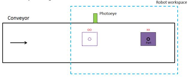
FIGURE 13 PART IS MOVED DOWNSTREAM USING CONVEYOR TO REPRESENT POINT XX
