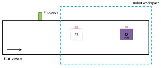
FIGURE 22 CONVEYOR MOVES PART DOWNSTREAM TO REPRESENT POINT XX
