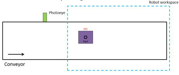
FIGURE 21 CONVEYOR MOVES PART DOWNSTREAM TO WITHIN ROBOT WORKSPACE TO REPRESENT POINT OO
