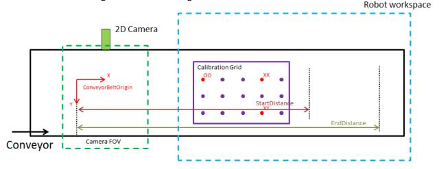
FIGURE 31 REPRESENTATION OF CONVEYOR TRACKING SETUP WHEN EXAMPLE IS FINISHED
