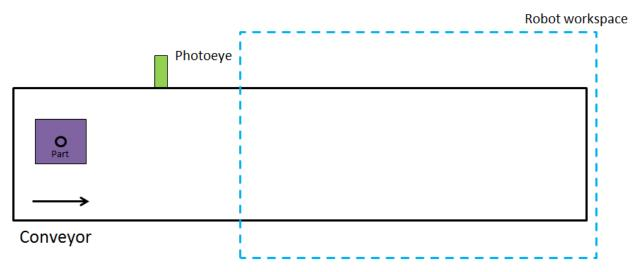
FIGURE 18 PART IS MOVING TOWARDS PHOTOEYE OUTSIDE OF ROBOT WORKSPACE
