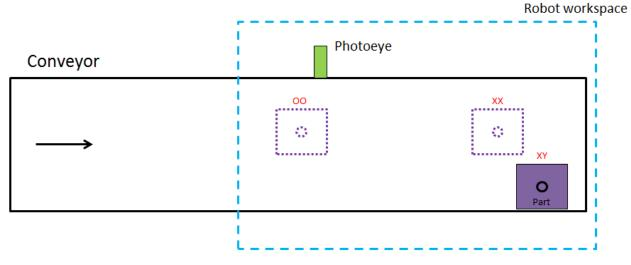
FIGURE 14 PART IS MOVED BY HAND TO DIFFERENT POSITION ON CONVEYOR TO REPRESENT POINT XY
