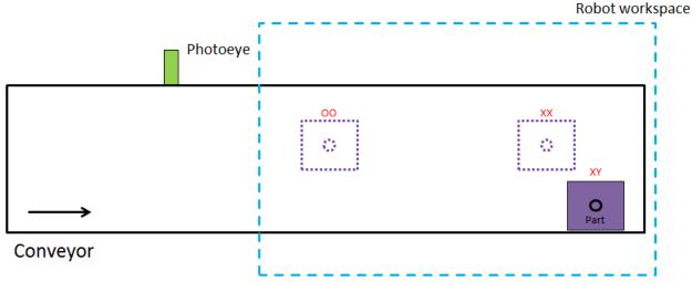
FIGURE 23 PART IS MOVED BY HAND TO NEW POSITION ON CONVEYOR TO REPRESENT POINT XY
