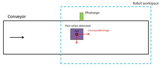
FIGURE 16 REPRESENTATION OF PART WHEN IT TRIGGERS PHOTOEYE. INITIALOBJECTPOSITION IN THIS SET UP IS [0 0 0 0 0 0]
