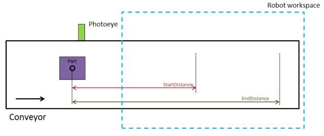
FIGURE 20 MEASUREMENTS OF STARTDISTANCE AND ENDDISTANCE
