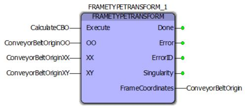
FIGURE 15 FUNCTION BLOCK IN MATH\_TOOLBOX TO CALCULATE A FRAME USING OO, XX, AND XY
