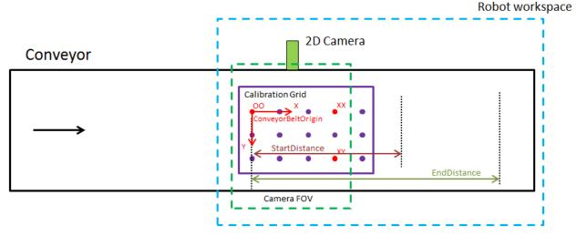
FIGURE 26 REPRESENTATION OF CONVEYOR TRACKING SETUP WHEN EXAMPLE IS FINISHED
