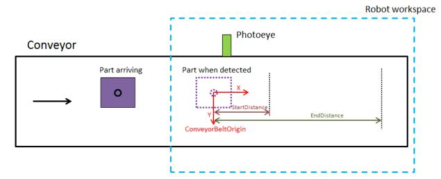
FIGURE 9 REPRESENTATION OF CONVEYOR TRACKING SET UP WHEN EXAMPLE IS FINISHED
