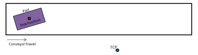
FIGURE 3 START OF PICK AND PLACE SEQUENCE, TCP STARTING FROM SAFE POSITION
