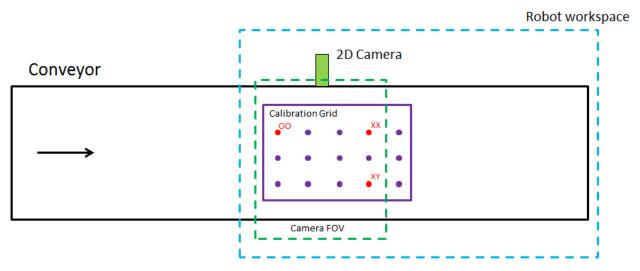
FIGURE 29 CALIBRATION GRID AND REPRESENTATION OF POINT XX AND XY
