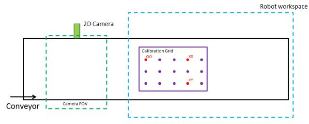
FIGURE 34 CONVEYOR IS MOVED DOWNSTREAM UNTIL OO XX XY ARE WITHIN ROBOT WORKSPACE
