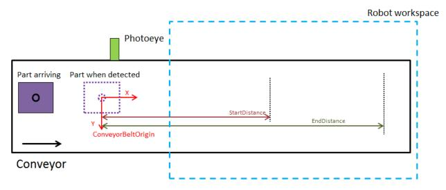
FIGURE 17 REPRESENTATION OF CONVEYOR TRACKING SETUP WHEN EXAMPLE IS FINISHED
