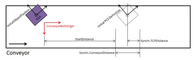
FIGURE 36 INITIAL DEFINITION OF PCS WHEN EXECUTIONMODE IS SATISFIED
