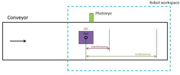
FIGURE 12 MEASUREMENTS OF STARTDISTANCE AND ENDDISTANCE
