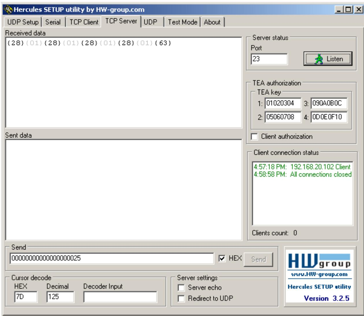
If you want to test the receiving portion of the Android application you can use the "Send" box pictured (make sure HEX is checked) and send 10 bytes (therefore 20 individual hexadecimal digits). Unless you know how 32-bit floating point numbers are represented in hexadecimal you will either need to use a decimal to hexadecimal online conversion application or just enter all 0's for the two REAL values. You can, however, use
