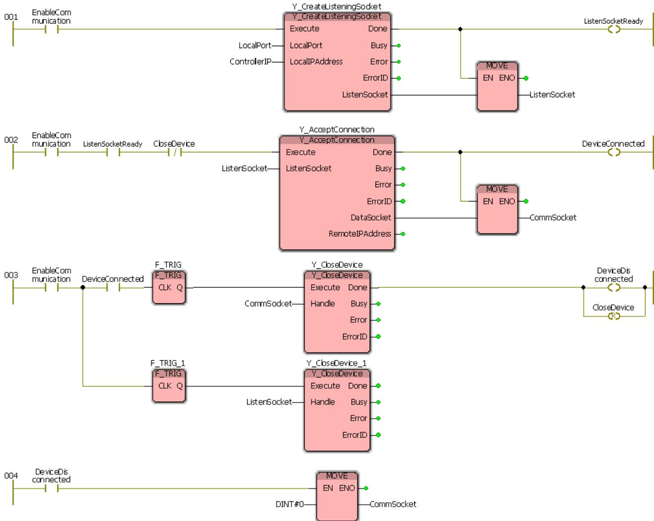
This methodology allows a single connection to be opened to the controller from a requester over port 23. It is important to note that the port number is independent of the application – you can choose the port number your controller and Android device communicate over, however it is suggested to avoid common port numbers associated with services like FTP, SMTP, etc. The above IEC code also handles a commanded disconnect that
