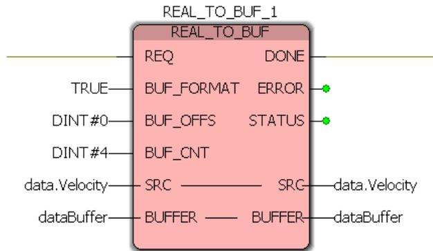
Setting *BUF\_FORMAT* to **TRUE** will ensure that the Android App properly interprets the input
