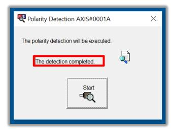
**Note:** If Pn080.1 (leading phase) is written to, Pn587 will need to be set to 1 to enable re-detecting polarity otherwise an A.C22 alarm will occur upon power cycle of the drive.
