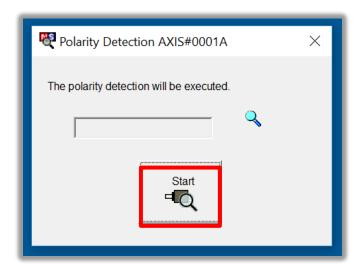
b. Cycle Power to the SERVOPACK after polarity detection has completed. If the motor is jogged before cycling power, an A.C22 alarm will appear after a power cycle and polarity detection will need to be executed again.
