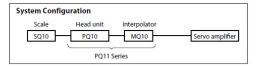
The encoder cable that connects the SmartScale Interpolator (MQ10) to the Yaskawa SERVOPACK must first be created by the user. The following components are needed to make this cable:
