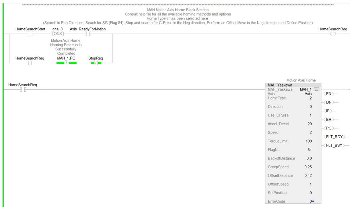
To start the homing search, the code is looking for the rising edge of either the HomeSearchStart bit or Input S12 from the amplifier I/O. As long as Axis\_ReadyForMotion is also true, the HomeSearchReq bit will be latched in. It will hold the enable on to the MAH AOI. This will stay latched until the home search is complete (PC) or a stop has been issued. This type of latched enable signal is used for most of the motion AOIs.
