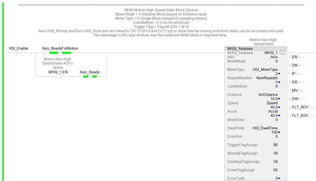
The code above uses a signal (HSI\_Enable or SI4) to enable the MHSI AOI. Using MHSI is a two-step process. It must be enabled for the trigger flag to start the index. There are many ways to adjust the move performed based on the inputs MoveMode, MoveType and CalcMethod.
