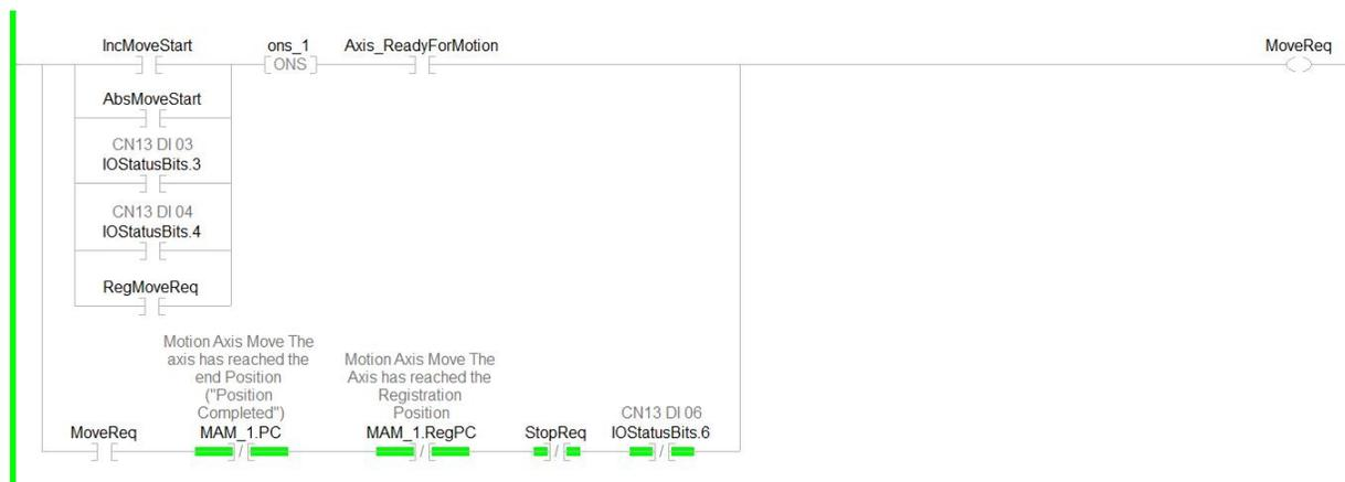
If the registration latch input is not activated, the motor will complete the original incremental or absolute index move and the PC output will turn on.
