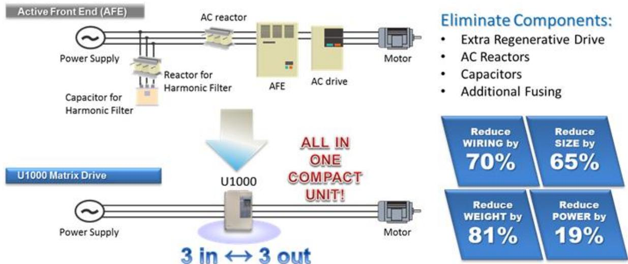
Compared to Yaskawa's classical solution (AC Drive with a regenerative front end), the U1000 Industrial Matrix Drive provides the same motor performance with these additional benefits:
