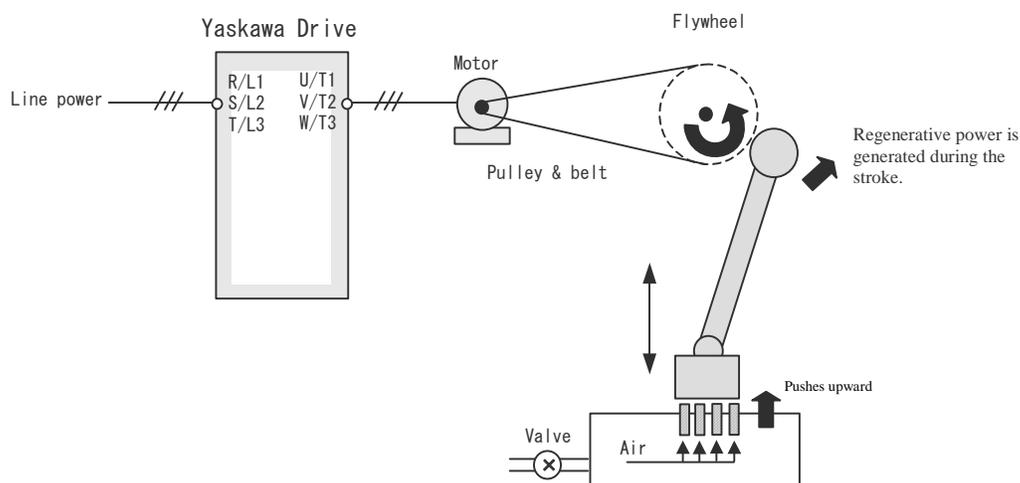
Drive adjustments provide a well-tuned motor and drive setup for flexibility, performance and extended machine, drive, and motor life. Acceleration and deceleration parameters enable the press to precisely control the operation to provide good electrical to mechanical power transfer. The Yaskawa drive allows for smooth accel and decel to reduce mechanical press wear.
