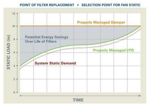
Figure 1 Design System Static<sup>2</sup>
