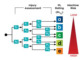
Yaskawa's FSoE servo amplifiers are capable of achieving PLe (equivalent to SIL3) which is suited for machines where serious injuries are possible, the frequency to exposure is long and/or frequent, and the possibility of avoiding injury is scarcely possible
