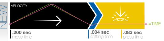
**220 parts/minute** = 3.676 parts/second = one part per .272 seconds
