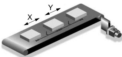
Frequently, a product at a particular point in a process arrives with non-repeatable, or random timing. In this application, a product needs to be placed on an exit conveyor with perfect spacing to ensure it can be wrapped and packaged accurately.
