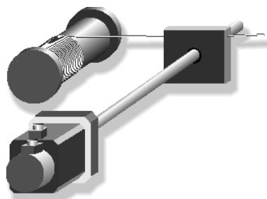
The product is wound onto a bobbin that rotates at a constant speed. The filament will be laid onto the bobbin by a ball screw driven guiding mechanism that will slowly decrease its travel rate as the winding diameter is increased.
