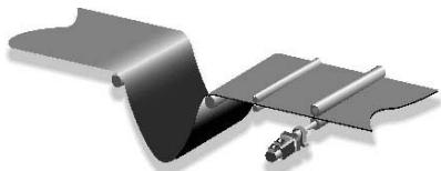
Many process lines that unwind a roll continuously and feed a converting process in discrete moves use an MP940. The servo feeds a variable length of material to the process and can include an optional external encoder to compensate for material slippage. In addition, an MP940 analog output varies the speed of the unwind roll as the depth of the material accumulator and the diameter of the unwind roll changes.
