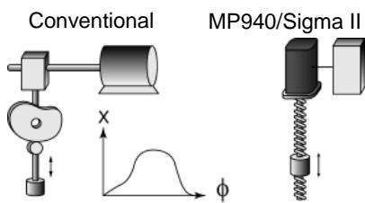
Machines that previously required mechanical cam changes for product or process changes may now be settable and reconfigured electronically. The servomotor is linked to a master encoder with synchronized phase control mode. With synchronized phase control mode, the AC servo system moves the same way as with a mechanical cam.
