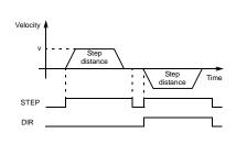
STEP bit: Refer to the Move Command message format, byte 2, bit 4.
