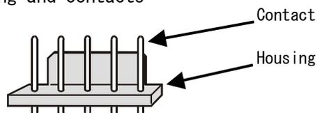
[Component Part Example 2] Switches, relays, and other parts with mechanical components
