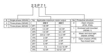
Note: Model Number and Drive Spec Number are required to fully define a drive.
