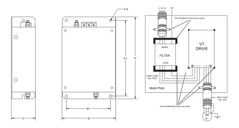
Figure 1-4. Installation of Line Filter and V7N Drive
