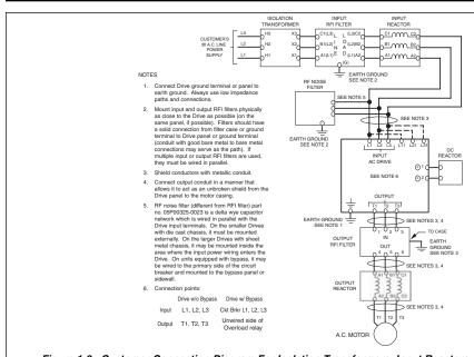
Figure 1-3. Customer Connection Diagram For Isolation Transformers, Input Reactors, Input RFI Filters,
