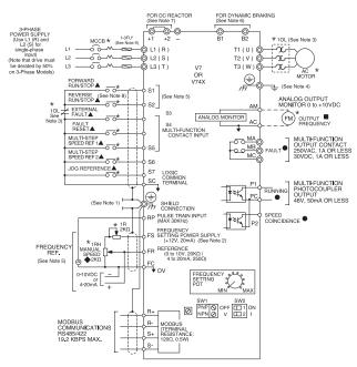
Figure 1-5. Standard Connections (2-Wire Control)
