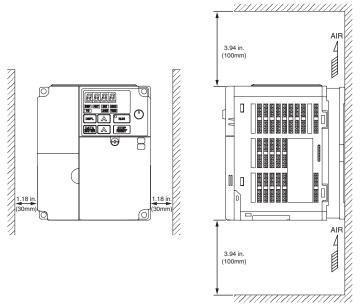
Important: To use the CIMR-V7\*U25P5, 27P5, 45P5, and 47P5 Drives as an open chassis, remove top and bottom covers and allow 1.97 in. (50mm) clearance on each side of the drive.
