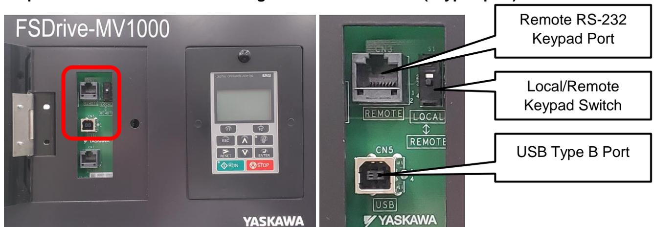
The MV1000 has two PC connection methods: USB (preferred) and Serial.
