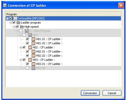
The CP ladder program with the check mark is converted. The ladder program cannot apply the check by disabling.
