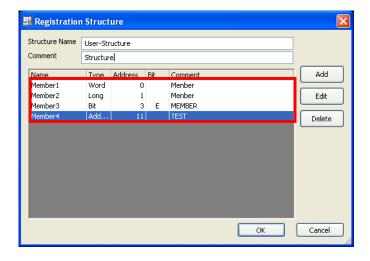
4. When "OK" in the "Registration Structure" dialog is pressed, the dialog is closed and the user structure is displayed in the variable sub-window.
