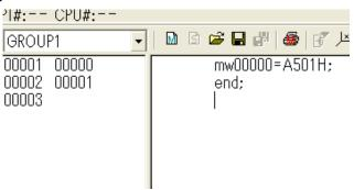
The register of ADDRESS type cannot be used in the motion main program. But, when "A501" was input by the hexadecimal number, this was judged the register of ADDRESS type.
