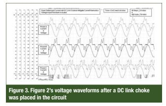
line reactors or DC link chokes. A line reactor is a set of three coils, one for each phase, placed in front of the VFD's diode bridge. The DC link choke is placed in the DC circuit of the drive just after the diode bridge. In the system represented in Figure 2, a DC link choke was available to be placed in the circuit so the effect on current distortion could be observed.
