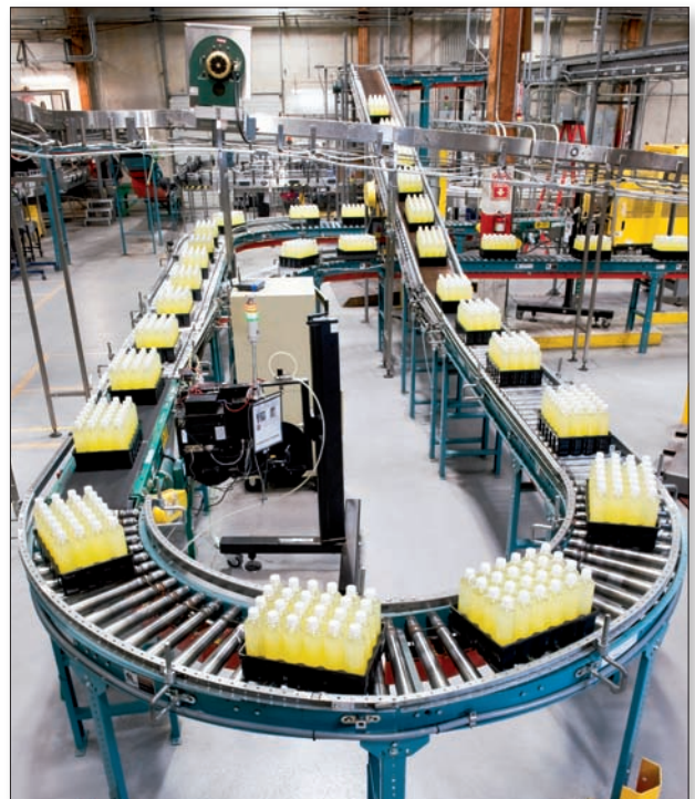
Depending on configuration and design, multiple motors can be used to share the load on conveyor belts such as this one moving bottles.
